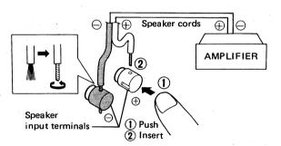
Depress the input terminal knob, insert the tip of the cord into the hole and then release the knob so that it springs back into position.
